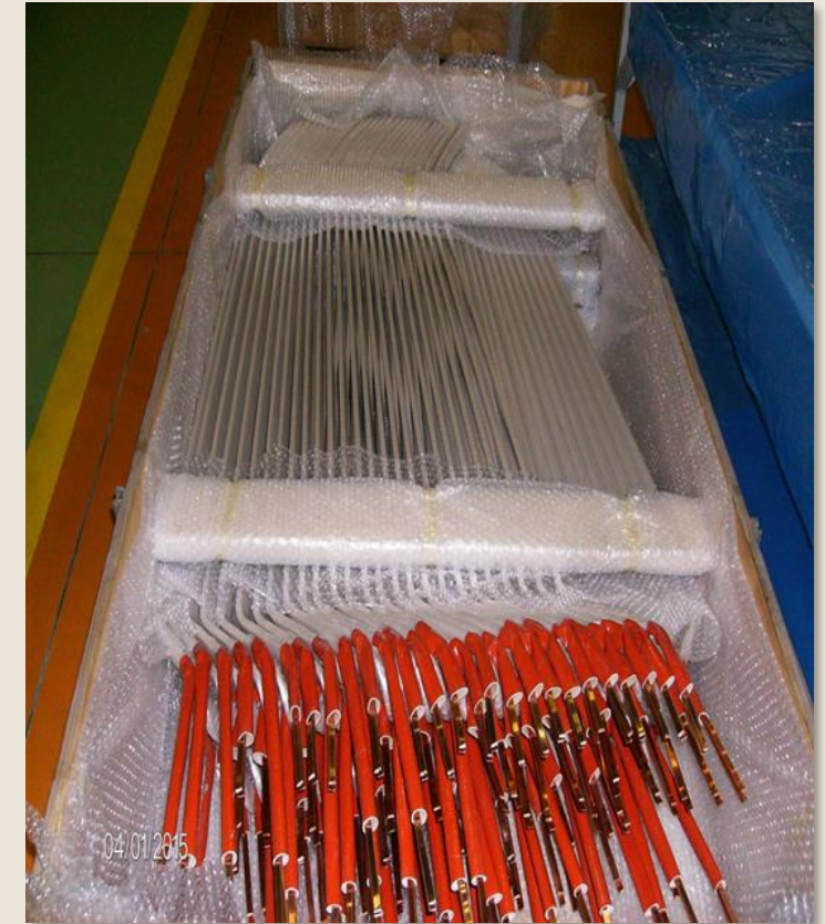
Coil set for stator windings
