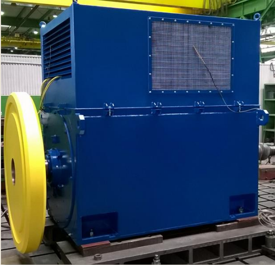
Type test of 1500 kVA, 6.6 kV, 600 rpm, IM B3, IC 01 Hydro generator
