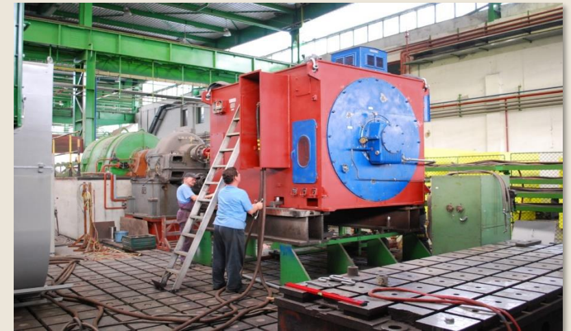
Type test (heat run test) of 4500 kW, 10 kV, 500 rpm, IM B3, IC 01 Cement mill asynchronous motor
