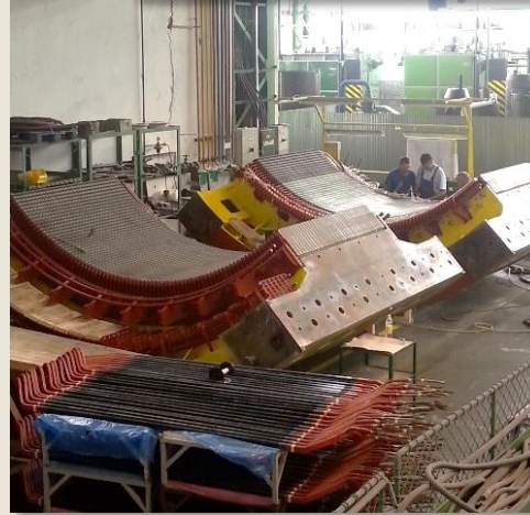
48,9 MVA 10,5 kV 250 rpm Hydro generator new stator laminated core manufacturing, rewinding Lajanuri HPP, Georgia
