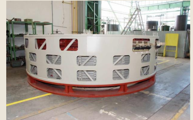
9,0 MVA 6,6 kV 250 rpm Hydro generator new stator housing & laminated core manufacturing, rewinding Rotor poles, bearings, brush system, brake refurbishment Gavünda, Sweden
