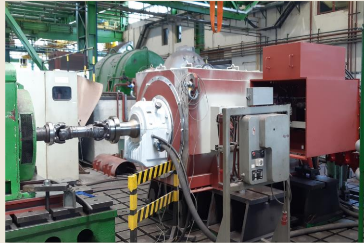
Type test of 3500 kVA, 11 kV, 1500 rpm, IM B3, IC 31 Steam turbine generator
