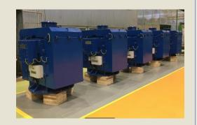
Slipring rotor induction machines
