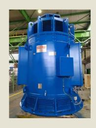
Salient pole synchronous machines
